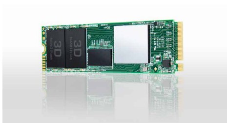
PCIe Gen3 x4 interface and NVMe standard
